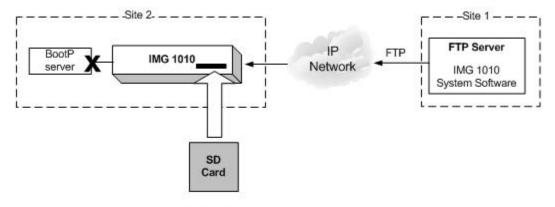
Bootup.cfg Host Flag = Retrieve IMG 1010 System Software from FTP server Server Address = Your FTP Server address
